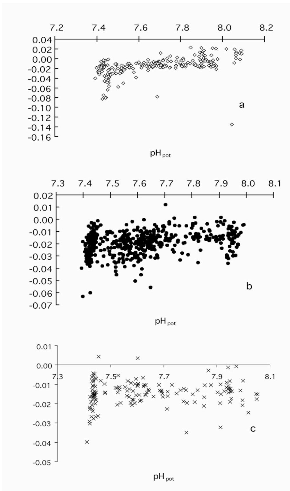
Fig.7.1. Difference of potentiometric and spectrophotometric methods for pH measurement; a - running pipette is used for spectrophotometric method; b - pHspec were obtained not using the running pipette; c -indicator and sample were mixed without air bubbles.
