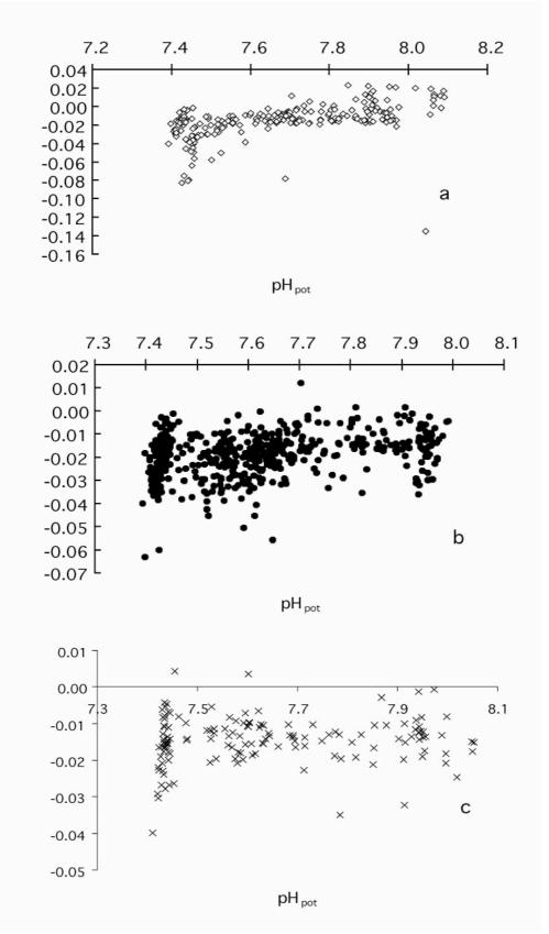
Fig.7.1. Difference of potentiometric and spectrophotometric methods for pH measurement; a - running pipette is used for spectrophotometric method; b - pHspec were obtained not using the running pipette; c –indicator and sample were mixed without air bubbles.
