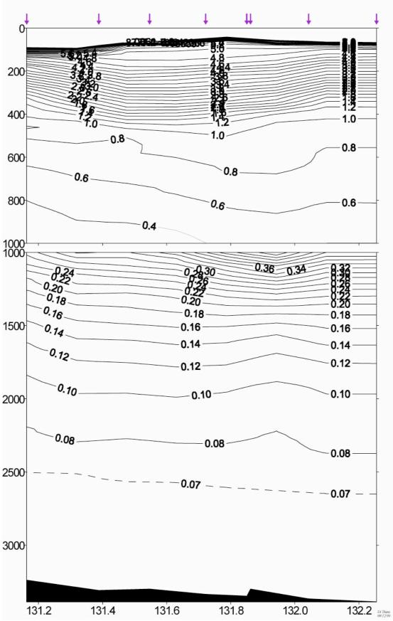
Fig. 9.7. Distribution of potential temperature on the section along 40°45'N, crossing the anticyclonic eddy 2, stations 188-194.
